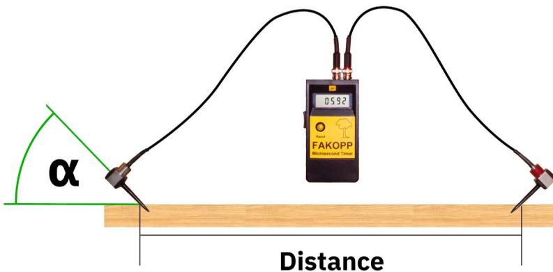
The angle of the needle has some effect on the transit time. We recommend an angle between 30°-60°, but never greater than 60°. Above 60° the readout is not reliable.
